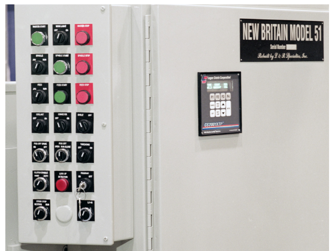
View of a CS2001XTP on a Model 51 New Britain. Works in conjunction with your existing push-button station.
