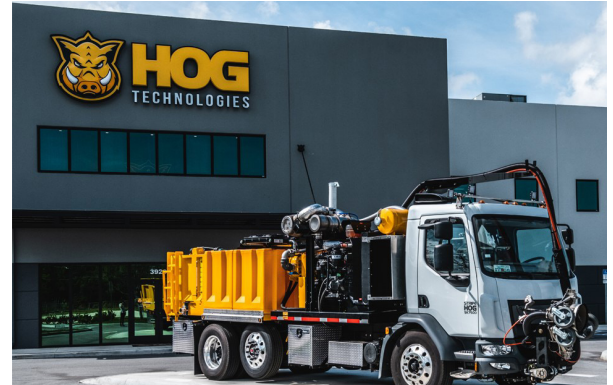
The Hog SK7500 uses an auxiliary engine with a Logan Bell-housing PTO clutch to power its waterblasting system
