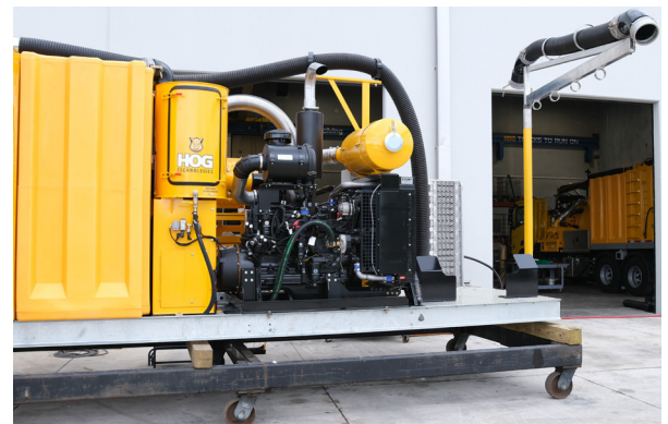
One of Hog’s SK3000 skid-mounted waterblasting systems with a Logan Bell-housing PTO clutch
