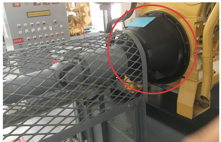
The Logan LC318 Bell-Housing PTO clutch fits in the same size envelope as the mechanical clutches. Available in pneumatically or hydraulically actuated, the LC318 can be engaged with push-button controls.
