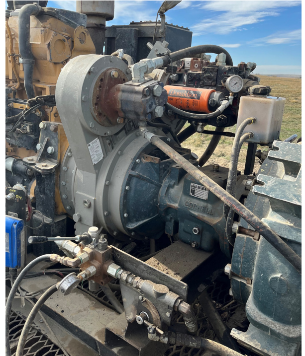
The Logan FlexaDrive is sandwiched between a CAT C15 engine and a Cornell 6819MP pump. Two PTO towers provide power to hydraulic pumps and other auxiliary equipment
