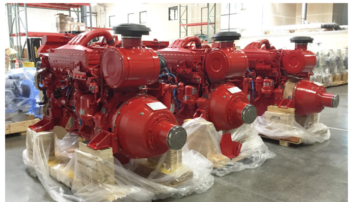
Cummins QSK 19-M Engines equipped with Logan LC-318 Bell Housing PTO's awaiting installation on to the San Francisco Fireboat St. Francis
